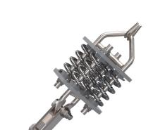
Reinforced stainless steel energy absorber with clevis, installed at one end of the lifeline, reduces stress in case of fall.
