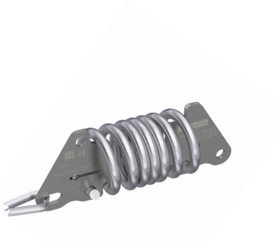
REF : 102173 Aluminium/stainless steel eye shock absorber, installed at one end of the lifeline, reduces stress on the structure in case of a fall. Traceability by unique serial number. Equipped with a tension and fall indicator.
